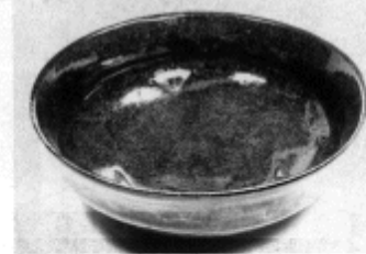
In strong sunlight, this sample of an aventurine glaze sparkles with gold flecks—minute crystals reflecting light from their faceted, mirrorlike surfaces.
